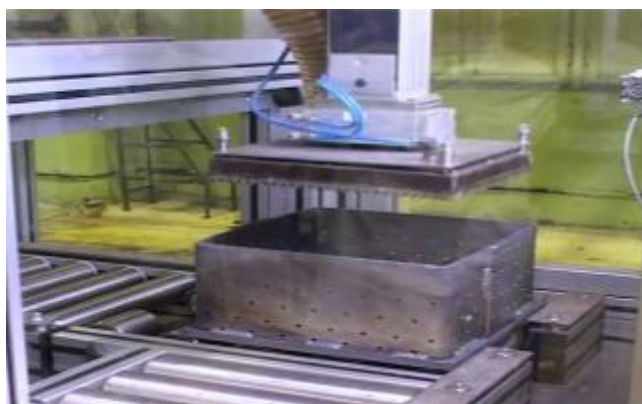
Stacker of pressed pellets in trough for sintering
