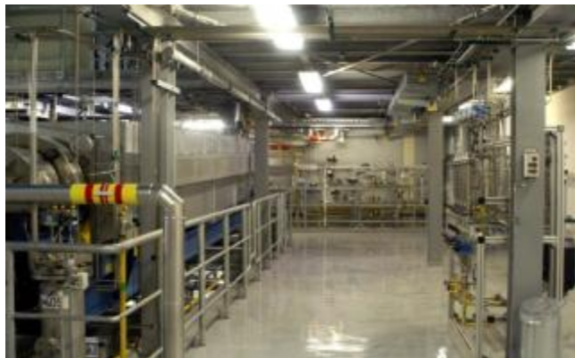
Section of uranium dioxide powder production by dry conversion technology
