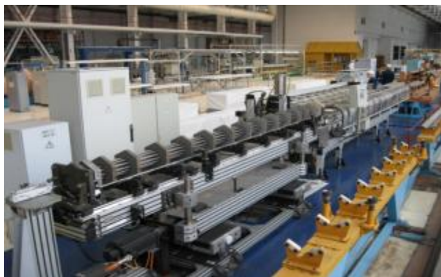
Automated bench for fuel bundle assembly
