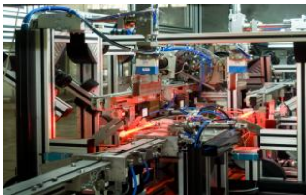
Equipment for optical inspection of pellets appearance
